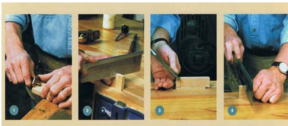
Picture No 21. Box Building with Lap Joints and Rabbets
